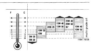
Recommended viscosity grades according to SAE at constant ambient temperatures
