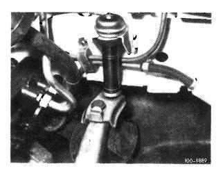
Type 115,114 Engine shock absorber left (straight-ahead)
