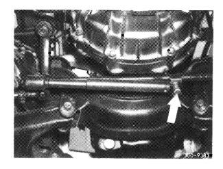
15 On type 123.1, unscrew engine bearer bolts at engine mount front, doing so from below. On type 115.1, work from above.
