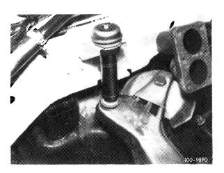
Type 115.114 Engine shock absorber right (straight-ahead)
